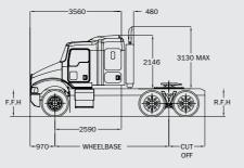
All frame height dimensions are to the top of the frame using 270mm rails.
